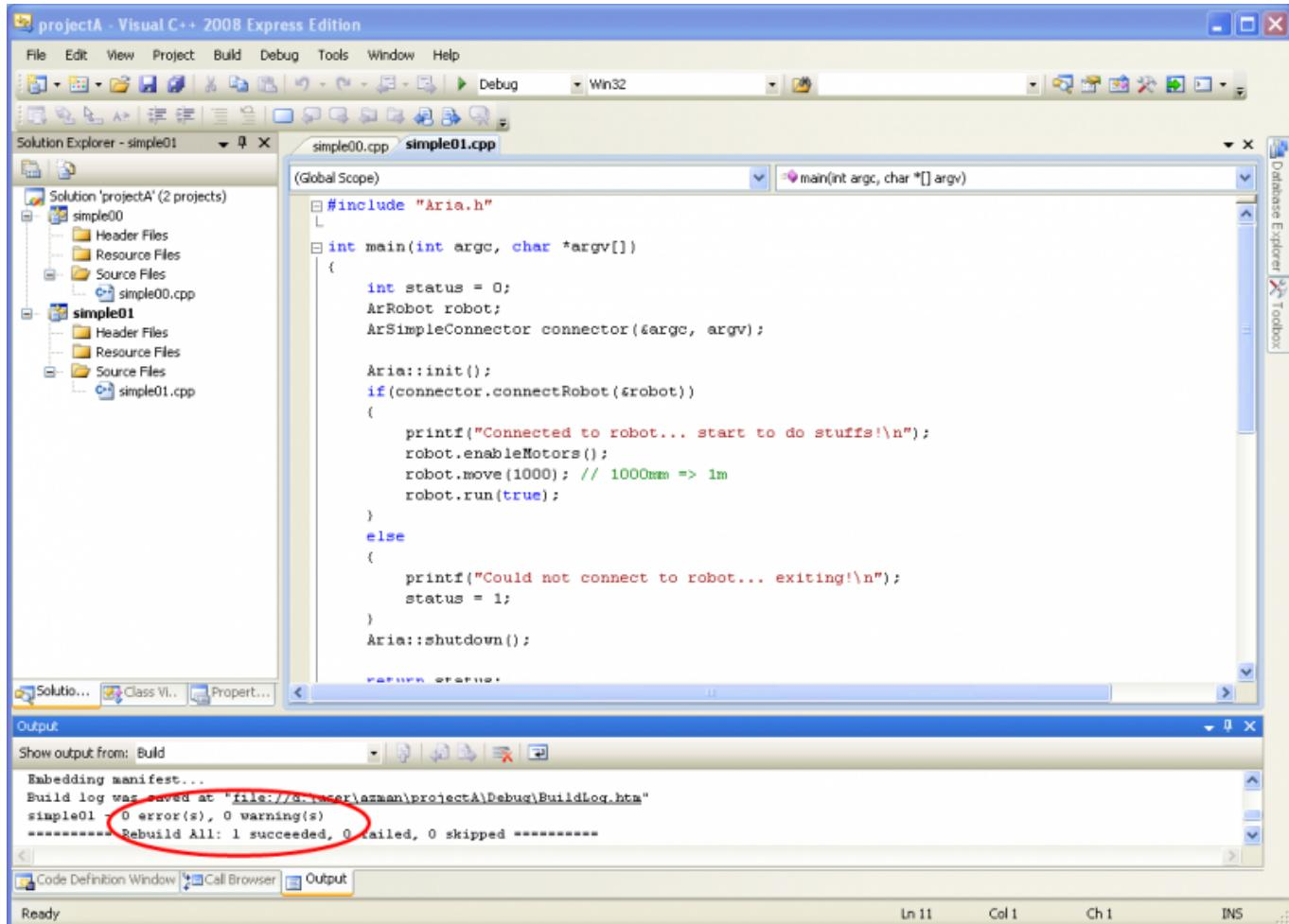
The distance argument for move method is in mm (millimeters). So, in the given code, we want to move the robot 1 meter forward. So how do we test this? Two options: (1) Run the program on a real robot, OR (2) Execute it in a simulator. Obviously, if we're testing miscellaneous things, going for the real robot is simply a hassle (that robot is quite heavy!). So, for this session we're going to go for the simulator approach.
