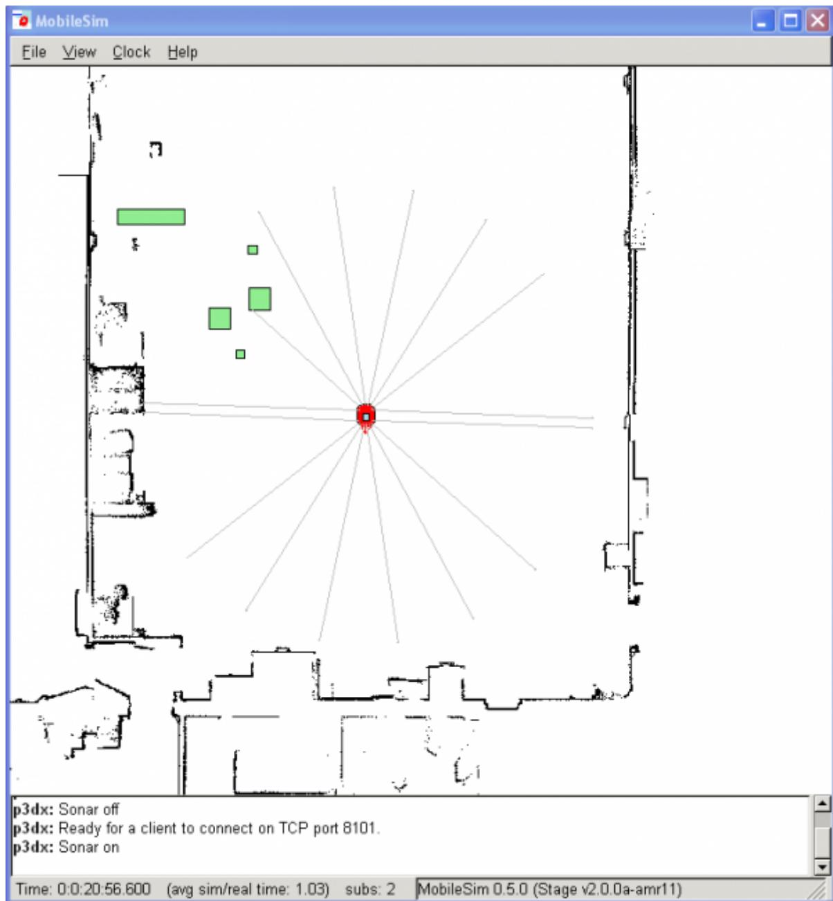
So, theoretically, you can start writing a program with any robot navigation algorithm that you know and try it here in this simulator. Obviously, your sensors/input are 'limited' (but Pioneer has a lot!) to what you have. You can, of course, create generic sensor devices but then it will not be 'practical'.
