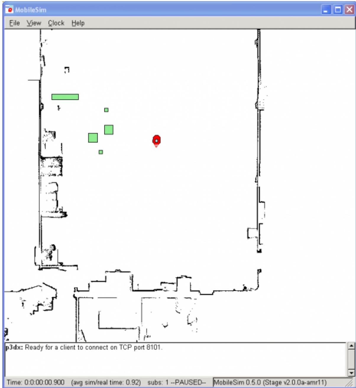
You'll see that the simulator waits for a client robot to connect to it using TCP port 8101 (this is the default).
