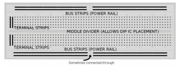
Notice the middle divider provides a way to place DIP ICs on the board, which is very useful for digital circuits.
