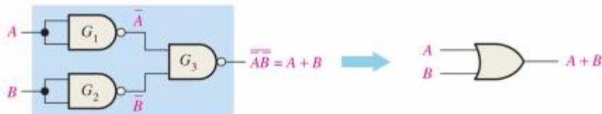
(c) Three NAND gates used as an OR gate
