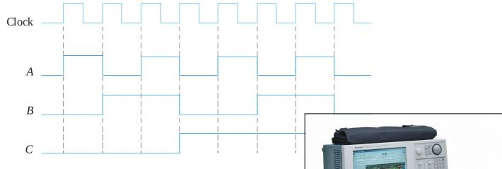
A diagram like this can be observed directly on a logic analyzer.
