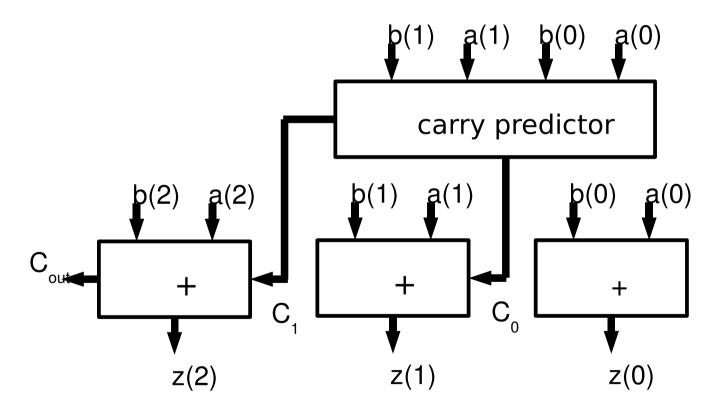
The carry bits can be generated with only 2 propagation delays (not 2n)
