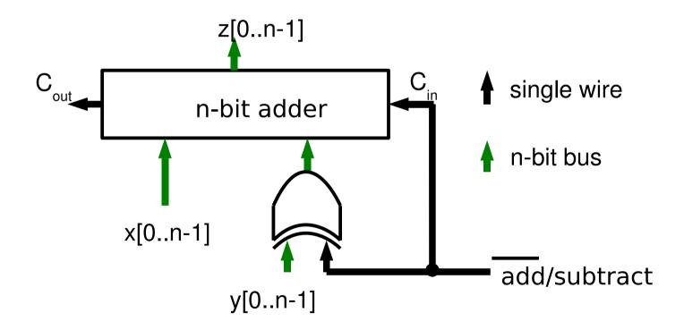
For this adder, can we use C<sub>out</sub> to set an overflow flag?
